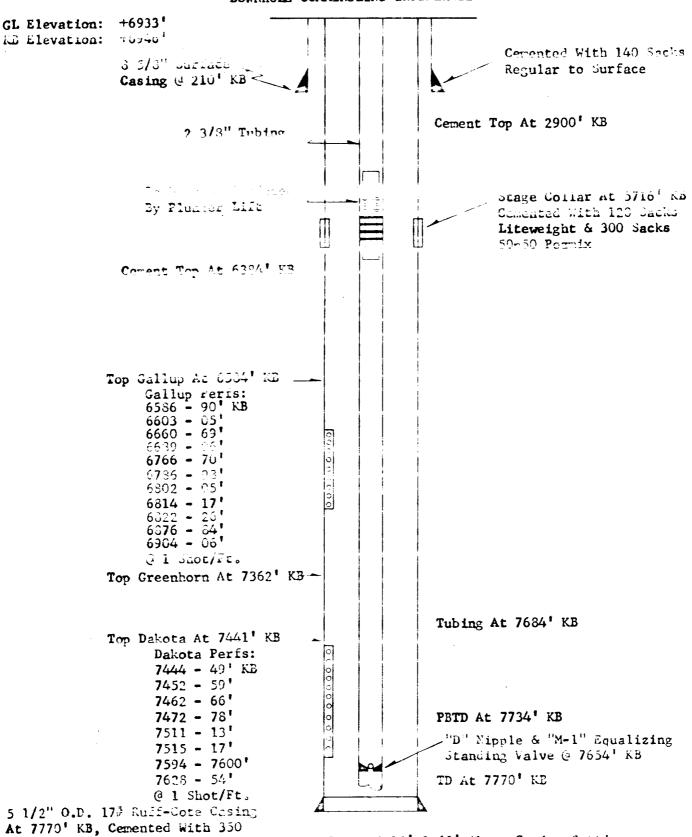
Sacks 50-50 Pozmix A Centralizers Located 10' & 60' Above Casing Setting Depth and 90' Thereafter to 6530' KE; Also One Centralizer 30' Above & 30' Below Stage Collar.
