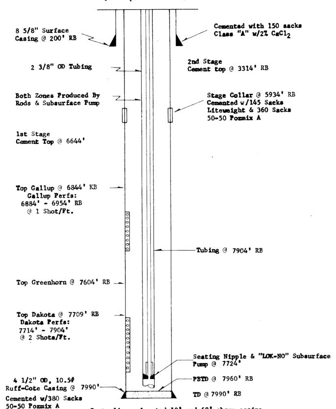
Centralizers located 10° and 60° above casing setting depth and 90° thereafter to 6500° RB; Also one centralizer 30° above and 30° below stage collar.
