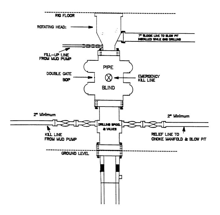
11" Bore, 2000psi minimum working pressure double gate BOP to be equipped with blind and pipe rams. A Schaffer Type 50 or equivalent rotating head to be installed on the top of the BOP. All equipment is 2000psi working pressure/or greater.
