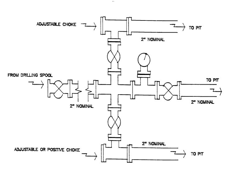
Minimum choke manifold installation from surface to Total Depth. 2" minimum, 2000psi working pressure equipment with two chokes.
