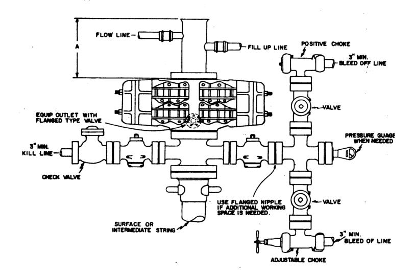
NOTE: BLOWOUT PREVENTER MUST HAVE DOUBLE RAMS; ONE BLIND & ONE PIPE RAM OR THE EQUIPMENT MUST CONSIST OF TWO BLOWOUT PREVENTERS. ONE EQUIPPED WITH BLIND RAMS & THE OTHER WITH PIPE RAMS. ALWAYS PLACE THE BLIND RAMS IN THE TOP PREVENTER.
