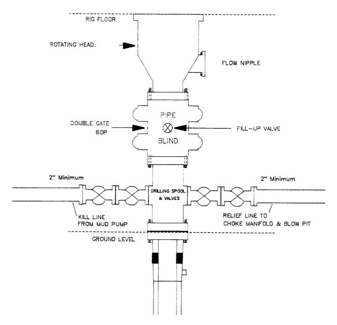
Minimum BOP installation for a typical Fruitland Coal well from surface to Intermediate casing point. 11" Bore (10" Nominal), 2000psi minimum working pressure double gate BOP to be equipped with blind and pipe rams. A Schaffer Type 50 equivalent rotating head to be installed on the top of BOP. All equipment is 2000psi working pressure/or greater.
