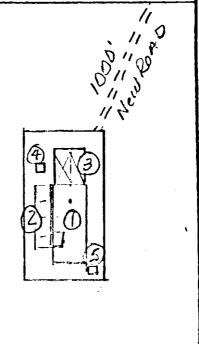
1. Rig 2. RESERVE Pit 56x25'x4' 3. Pipa Lincks 4. Compressor 5. The Pile P.
