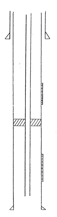
8-5/8", 24# casing set at 145', cemented with 125 sxs.
