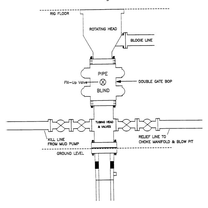
Minimum BOP installation for Completion Operations. 7 1/16" Bore (6" Nominal), 3000psi minimum working pressure double gate BOP to be equipped with blind and pipe rams.
