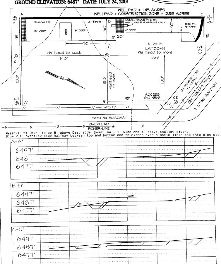
Note: Contractor should call One–Call for location of any marked or unmarked buried pipelines or cable: on well pad and/or access road at least two (2) working days prior to construction
