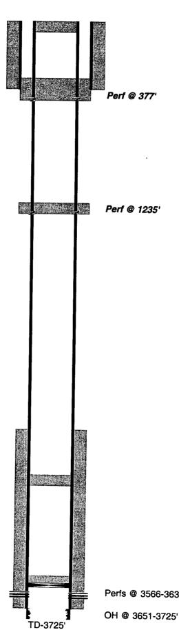
12-1/4" hole @ 327' 8-5/8" csg @ 327' w/300sx-TOC-Surf-Circ
