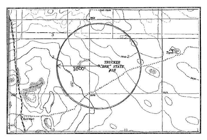
Assumed 100 ppm  $ROE = 3000^{\circ}$  100 ppm H2S concentration shall trigger activation of this plan.
