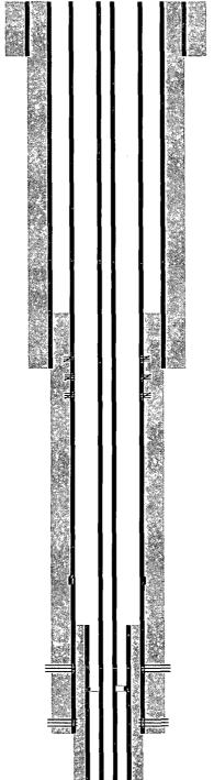
17-1/2" hole @ 469' 13-3/8" csg @ 469' w/ 475sx-TOC-Surf-Circ
