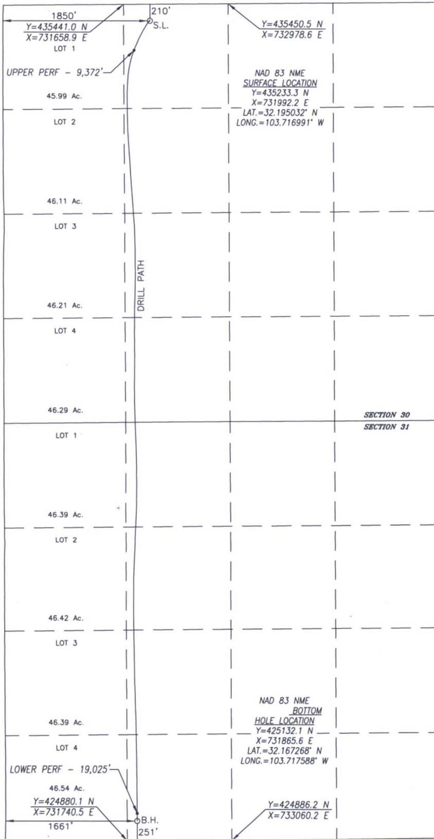
BOREPATH SHOWN HEREON IS BASED ON DIRECTIONAL SURVEY REPORT PROVIDED BY COG FOR THE WINDWARD FEDERAL #7H SUPPLIED TO HARCROW SURVEYING, LLC ON 9/27/17.
