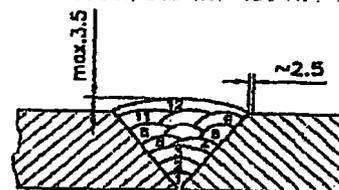
**Groove Design for Test Coupon**
