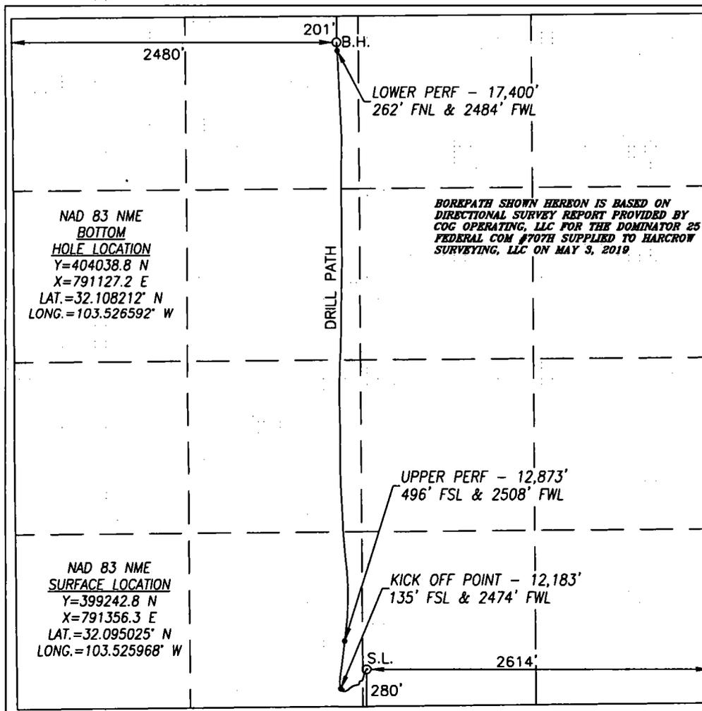
BOREPATH SHOWN HEREON IS BASED ON DIRECTIONAL SURVEY REPORT PROVIDED BY COG OPERATING, LLC FOR THE DOMINATOR 25 FEDERAL COM #707H SUPPLIED TO HARCROW SURVEYING, LLC ON MAY 3, 2019
