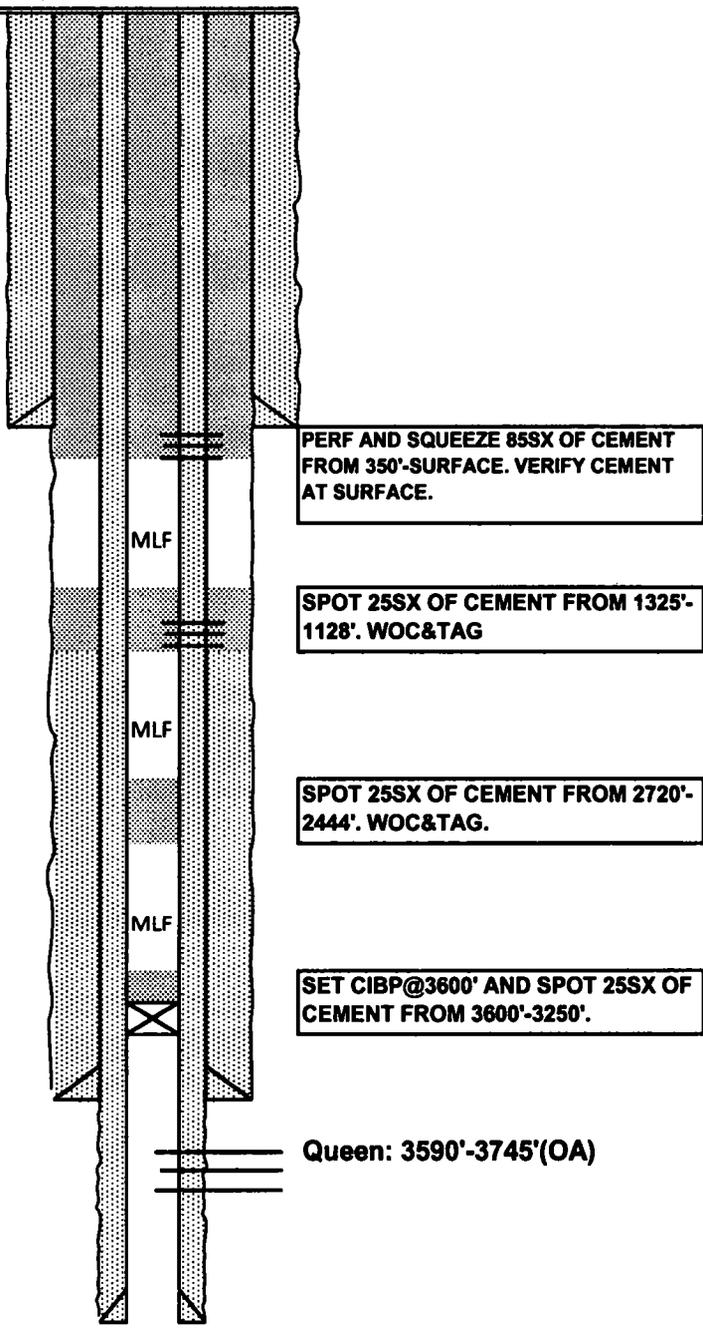
PERF AND SQUEEZE 85SX OF CEMENT FROM 350'-SURFACE. VERIFY CEMENT AT SURFACE.
