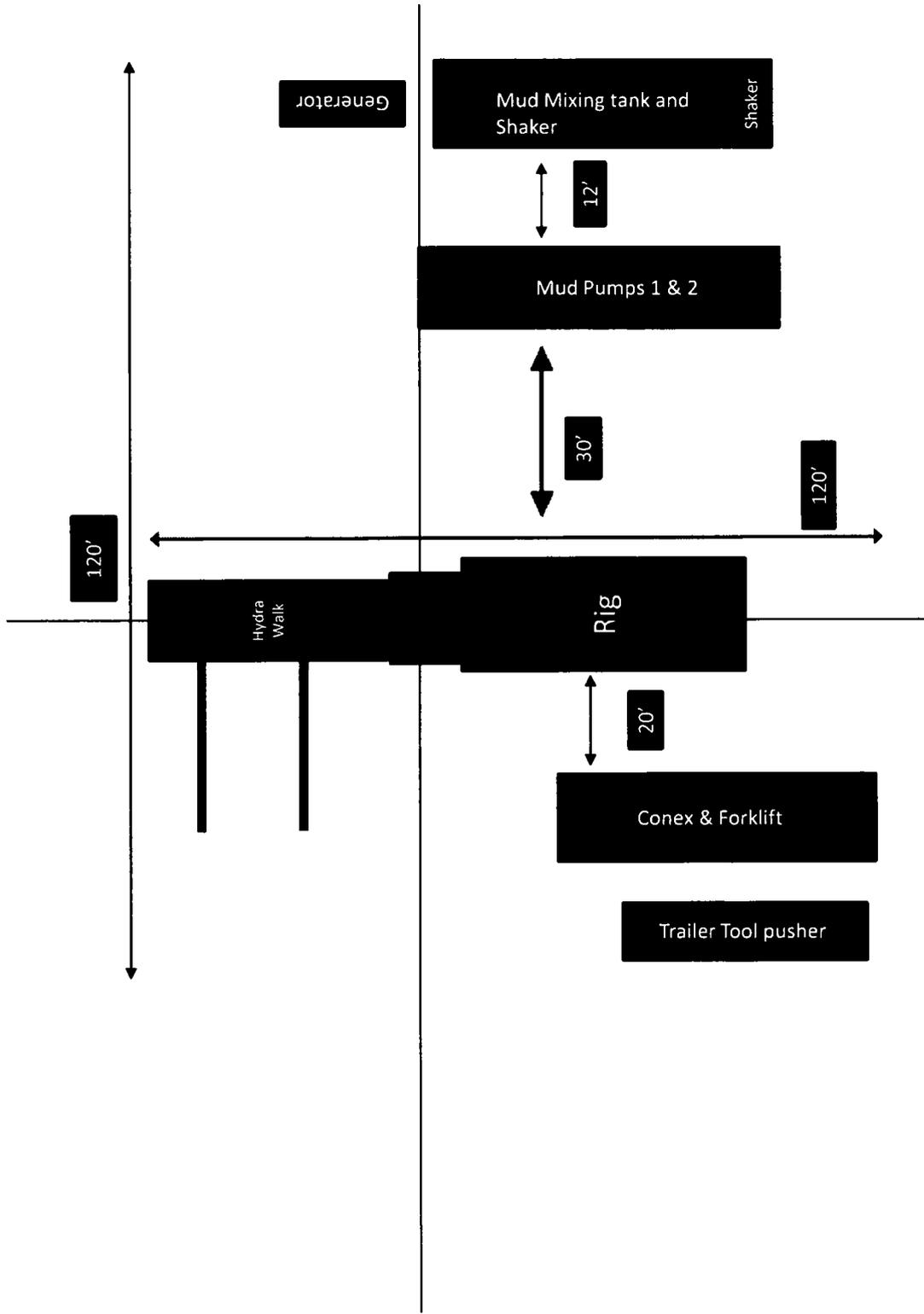
**OXY USA Inc. - Lost Tank 30-19 Federal Com 1H – Amended Drill Plan**
