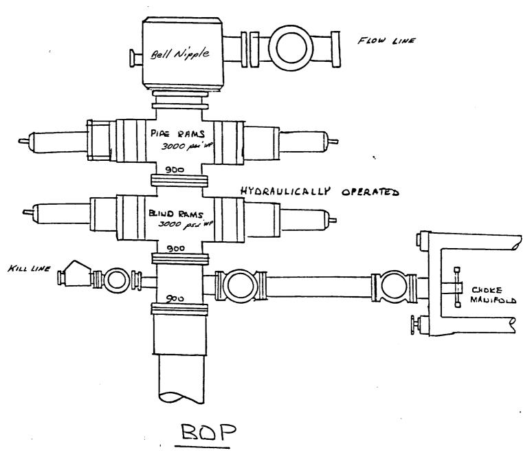
All additional valves and connections are the same working pressure.
