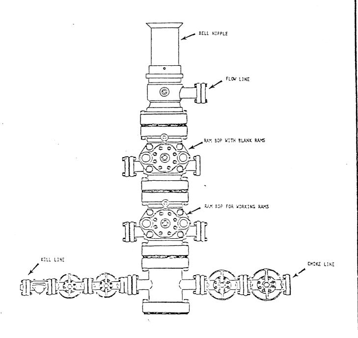
BOP rams will be actuated on each trip of drill pipe and will be tested before drilling the plug on each casing string.
