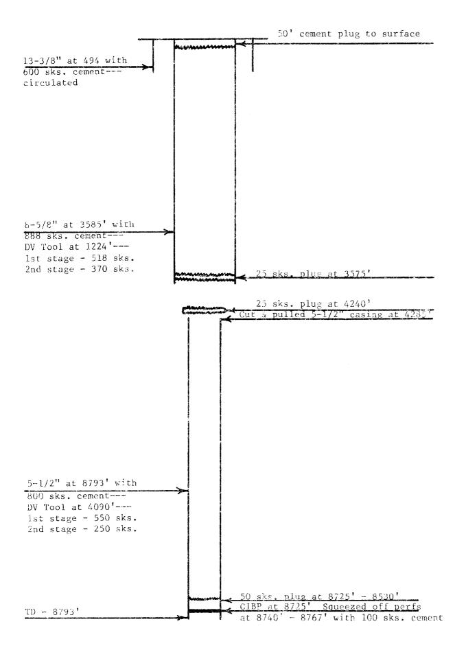
Well was originally drilled in 1956. Elevation - 3004 GL
