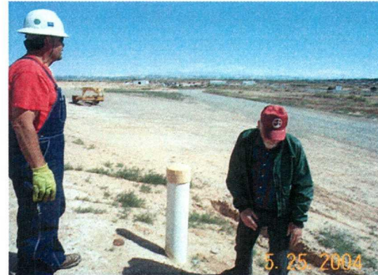
Skim pit leak detector-noted DRY.
