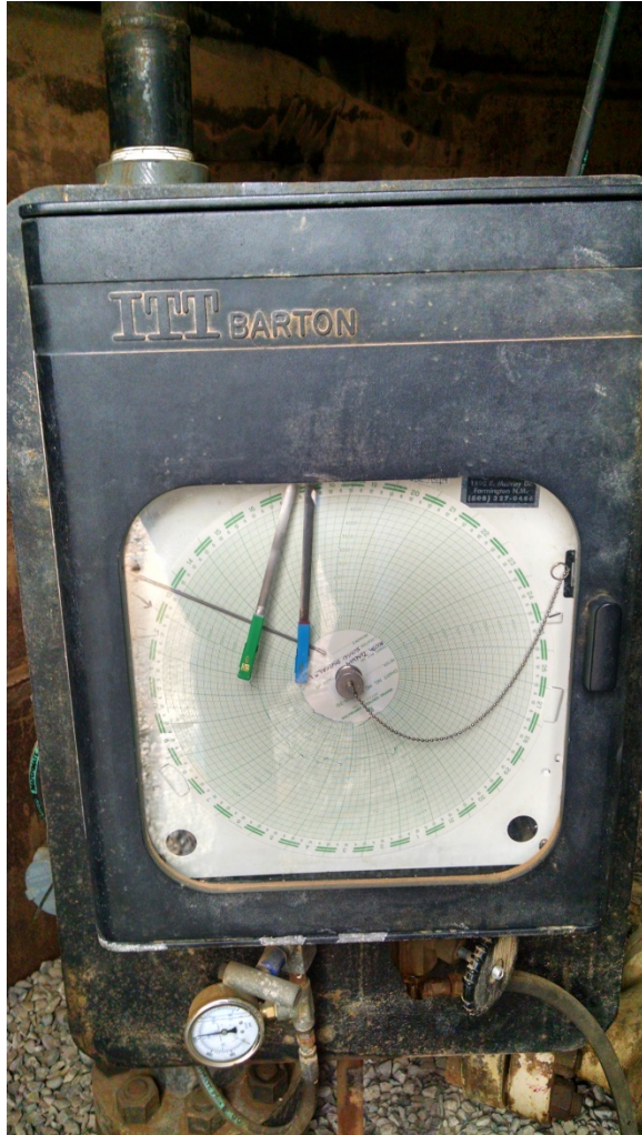
Pump turned on at ~ 167 bbls/hr at 1,800 psig well below MSIP of 2,400 psig
