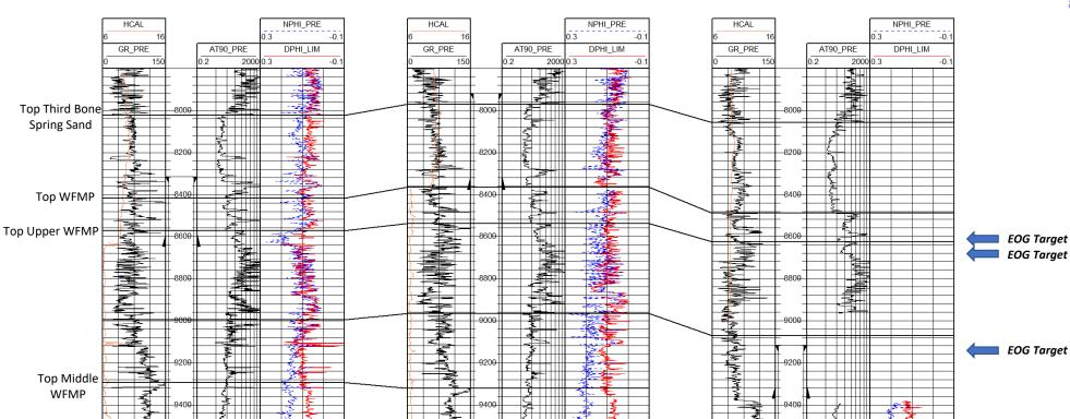
Log acronyms: GR/GRS/GRD: Gamma Ray HCAL: Caliper log AT90\_PRE: Resistivity NPHI\_PRE: Neutron Porosity DPHI\_LIM: Density Porosity NSP Notice List - Inga 33 Fed Com EOG Resources, Inc. EXHIBIT A- Notice List
