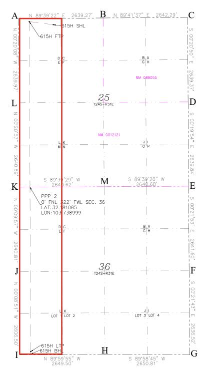
A=N:435400.07 E:724859.41 B=N:435415.91 E:727498.63 C=N:435430.04 E:730140.88 D=N:432790.73 E:730156.88 E=N:430150.93 E:730172.17 F=N:427509.39 E:730188.98 G=N:424872.92 E:730205.63 H=N:424871.96 E:727554.82 I=N:424871.01 E:724905.32 J=N:427478.51 E:724898.61 K=N:430119.30 E:724890.83 M=N:432760.15 E:724874.87 M=N:430135.06 E:727531.54 Non-Standard Location Application
