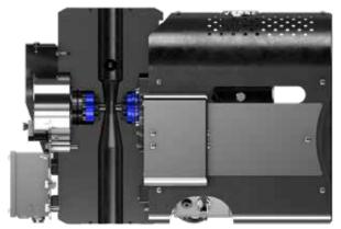
The Vx Spectra flowmeter contains a venturi section with multivariable transmitter for measuring total flow rate; a nuclear source and detector that obtain oil, gas, and water holdups; and a compact flow computer that performs all calculations and converts flow measurements from line to standard conditions.
