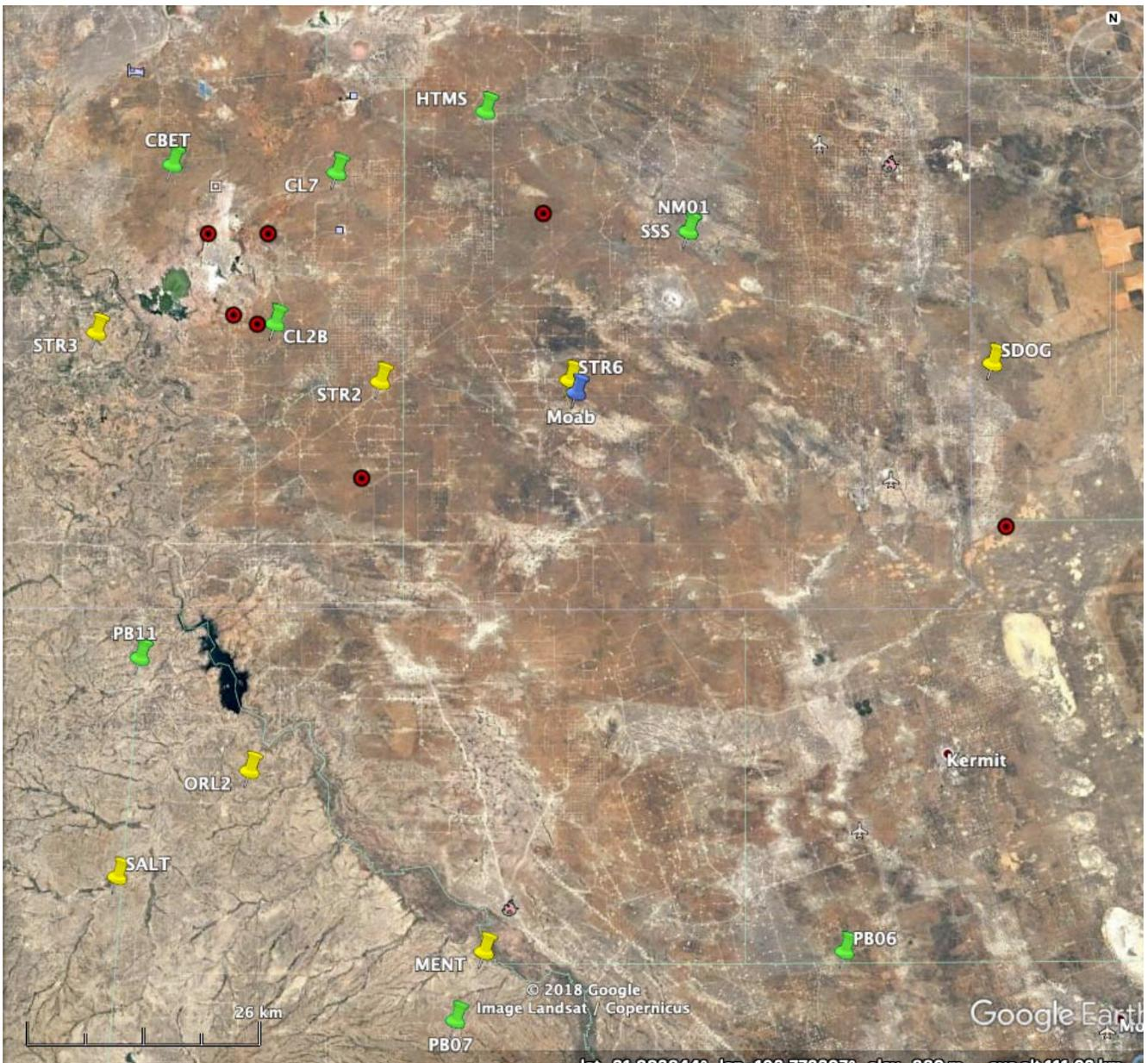
**Figure 2.** Striker SWD wells seismic station locations (yellow push pins) and existing NGL-Permian seismic stations (yellow pushpins). Other regional seismic stations run by TexNet and New Mexico Tech are shown as green pushpins. Historic seismicity listed in Table 1 shown as red circles. Moab SWD well shown as blue pushpin.
