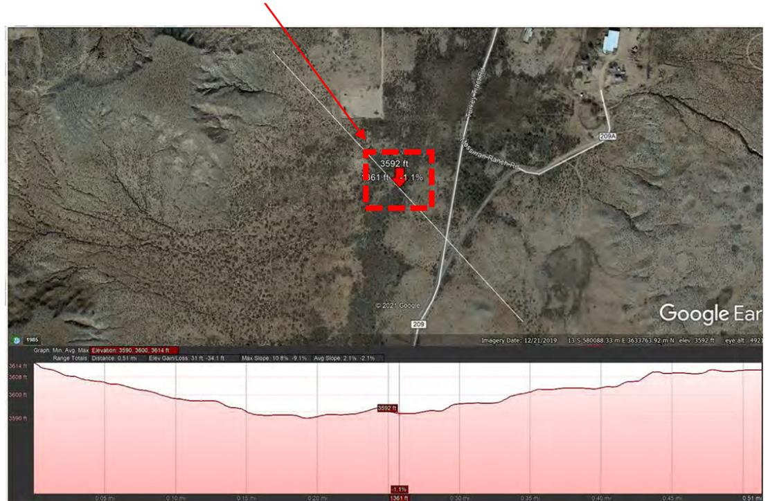
Spurs surface location does not contemplate the fact that it is in a natural water drainage area. This terrain is prone to flooding, which can lead to significant operational issues and added costs.
