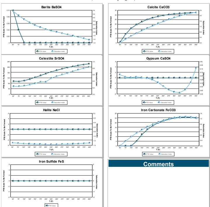
Scaling predictions calculated using Scale Soft Pitzer 2017
