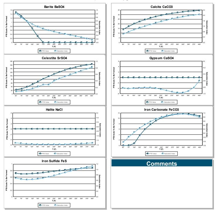
Scaling predictions calculated using Scale Soft Pitzer 2017
