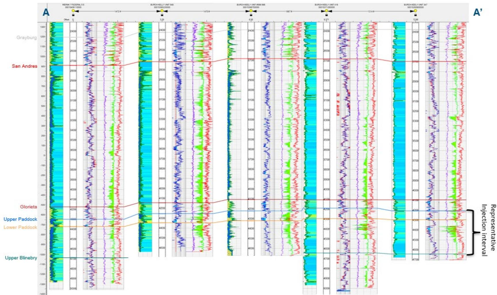
At the BKU #566, the top of the Yeso formation is at 4,207' and the perforated injection interval will be from 4,240' to 4,540'. The producing formation is well established as demonstrated by the associated cross section, and the nearby offset well Burch Keely Unit #416 (API# 30-015-37128) shows the top of the Yeso at 4,198' and the top of the underlying Blinebry formation at 4,640'.
