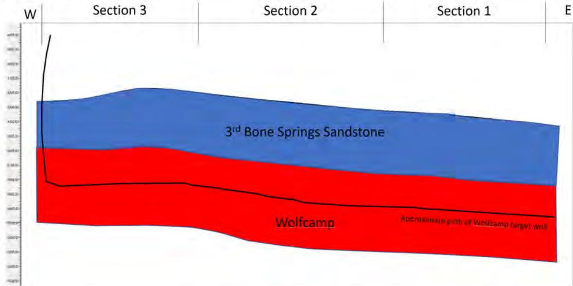
Exhibit B-6 is a generalized cross section with approximate well trajectory.
