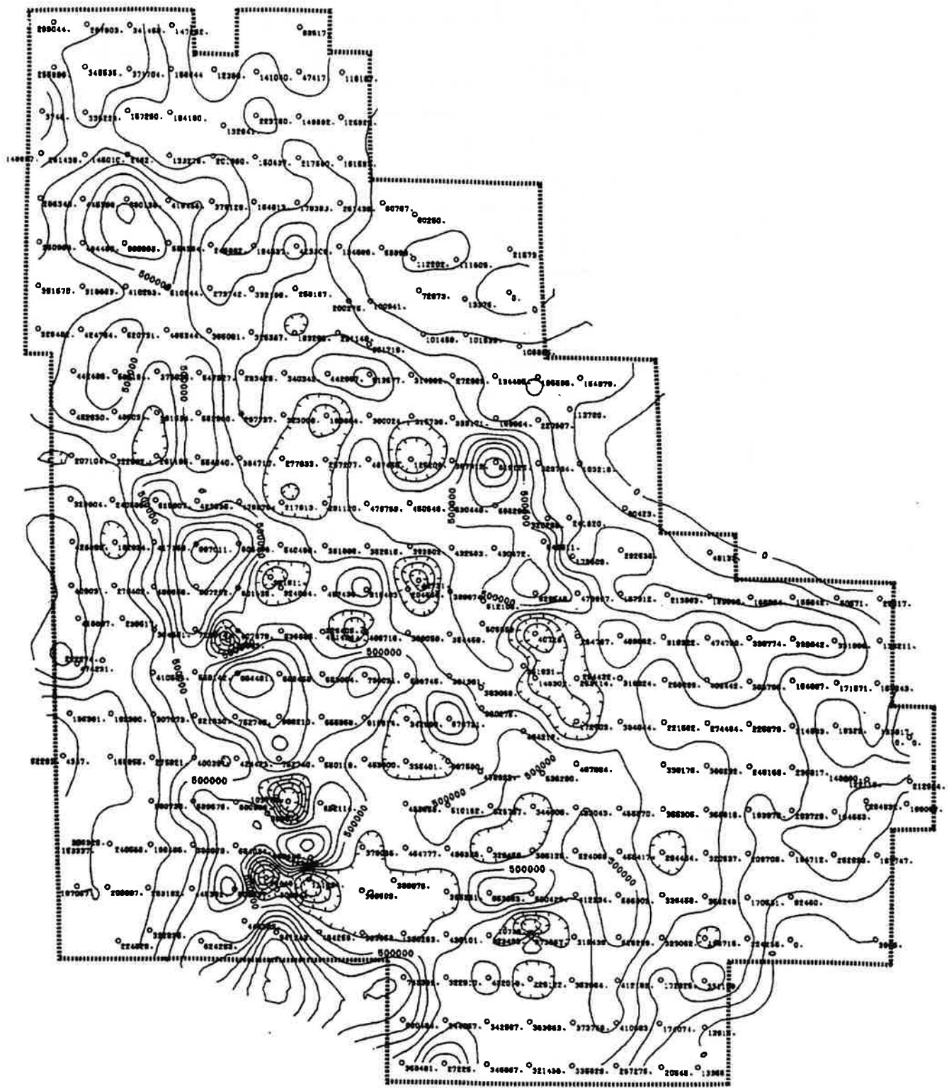
EUNICE MONUMENT SOUTH UNIT CONTOUR ON CUMULATIVE OIL PRODUCTION THROUGH 1981 CONTOUR INTERVAL = 100,000 STB SCALE: 1" = 4000'
