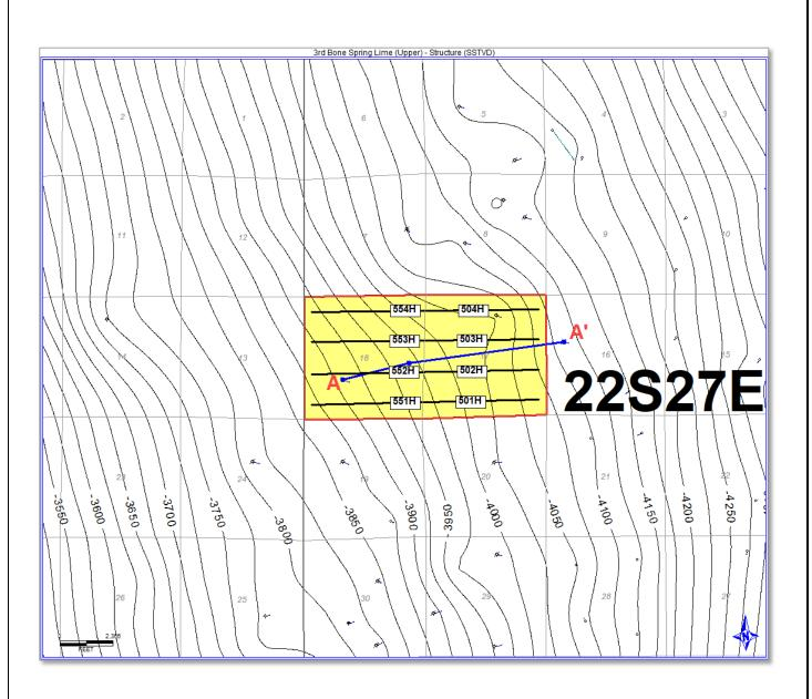
**Alpha Exhibit B-3** Cross-section A-A'. Stratigraphic cross-section hung on top of the 3<sup>rd</sup> Bone Spring Upper. 501H-504H target intervals (Second Bone Spring Sand Targets) indicated by the red arrow. 551H-554H target intervals (Harkey Sand Targets) indicated by the blue arrow.
