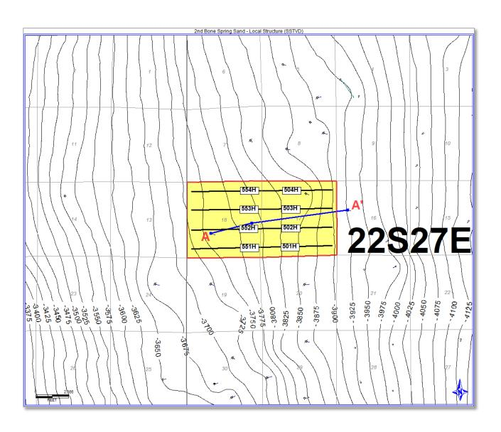
**Alpha Exhibit B-2** is a structure map showing the depth (subsea) to the top of the 3<sup>rd</sup> Bone Spring Carbonate (of which the Harkey Sandstone is a member), and the location of the proposed wells. The location of the west to east A-A' Cross-Section is also noted. Contour Interval is 25'.
