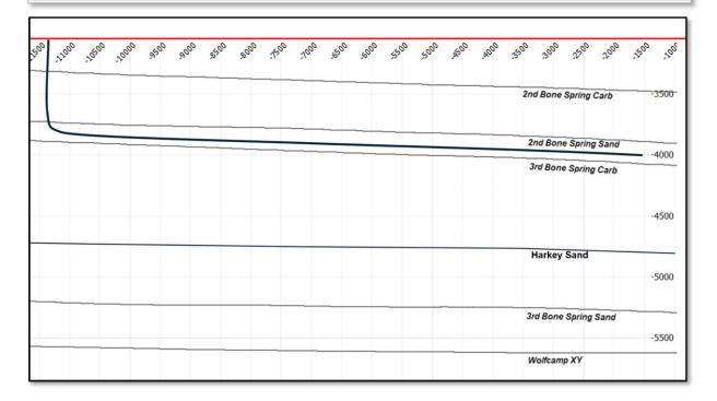
**Alpha Exhibit B-8** is a cross section with an approximate well trajectory representing the 551H-554H wellbores.
