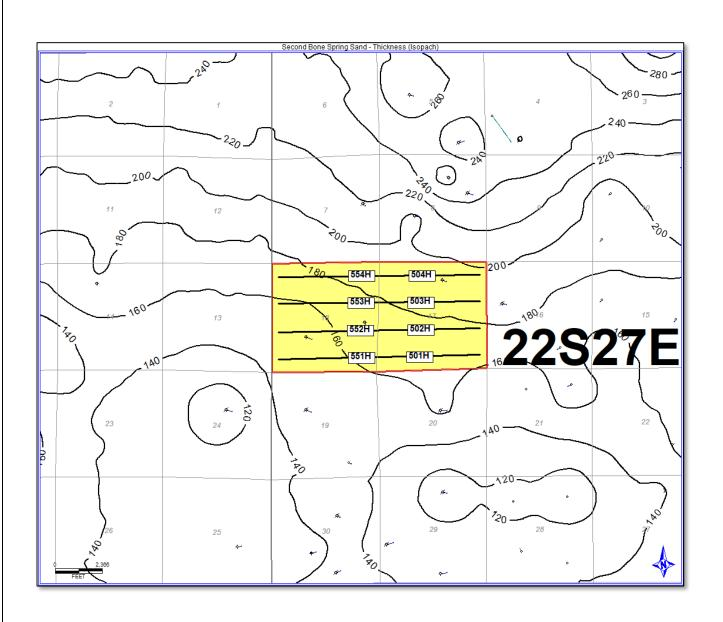
**Alpha Exhibit B-5** is a gross isochore of the 3<sup>rd</sup> Bone Spring Carbonate with a 20' contour interval. Map demonstrates continuity and consistent thickness of the target zone.
