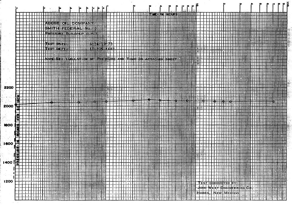
ADOBE OIL COMPANY SMITH FEDERAL No. 2 PRESSURE BUILD-UP TEST TABULATION OF PRESSURE AND TIME TEST CONDUCTED BY: JOHN WEST ENGINEERING CO.
