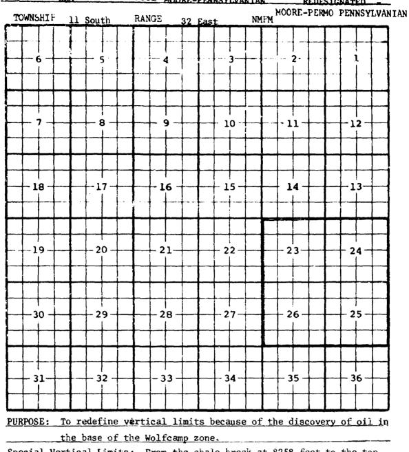
Special Vertical Limits: From the shale break at 8258 feet to the top of the Mississippian at 9974 feet as in Amerada Petroleum Corporation, State "MA" No. 1, located in Unit M of Section 24, Township 11 South, Range 32 East. Pool boundary colored in red. SECTION 23: All SECTION 24: All SECTION 25: All SECTION 26: All TO BE DISMISSED PENDING FURTHER STUDY.
