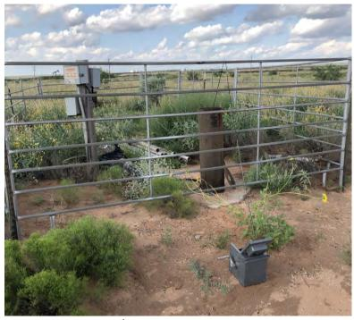
SP6 – Well USGS-9579/Misc. 161 where we were able to measure a depth to groundwater in abandoned casing near the well (32 16 12.85, -103 45 2.11).
