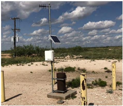
SP-7 Well C-2954/Misc. 428 is SNL-8, a WIPP monitoring well. Data for this well presented in this submission documents the fact that alluvial water is not present. (32 17 14.66, -103 47 53.53)
