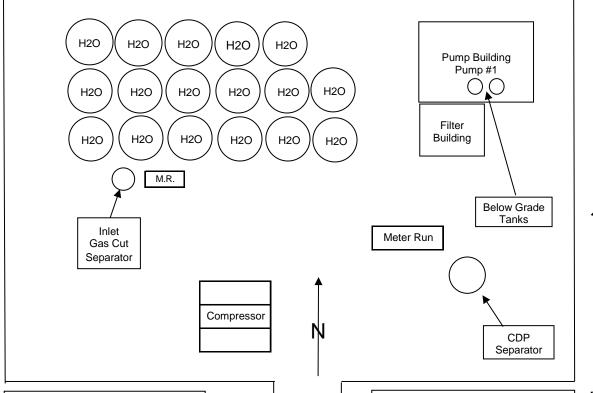
Inlet gas cut separator - PESCO 2 ph Vertical, 85,000 Btu/Hr SN -40025 Mfg - 1987 CDP Separator - PESCO 2 ph Vertical SN - 401959 Mfg - 1995 12" x 24" Catalytic Heater Filter Pots - 1 - SN 16686, 2 - SN 13287
