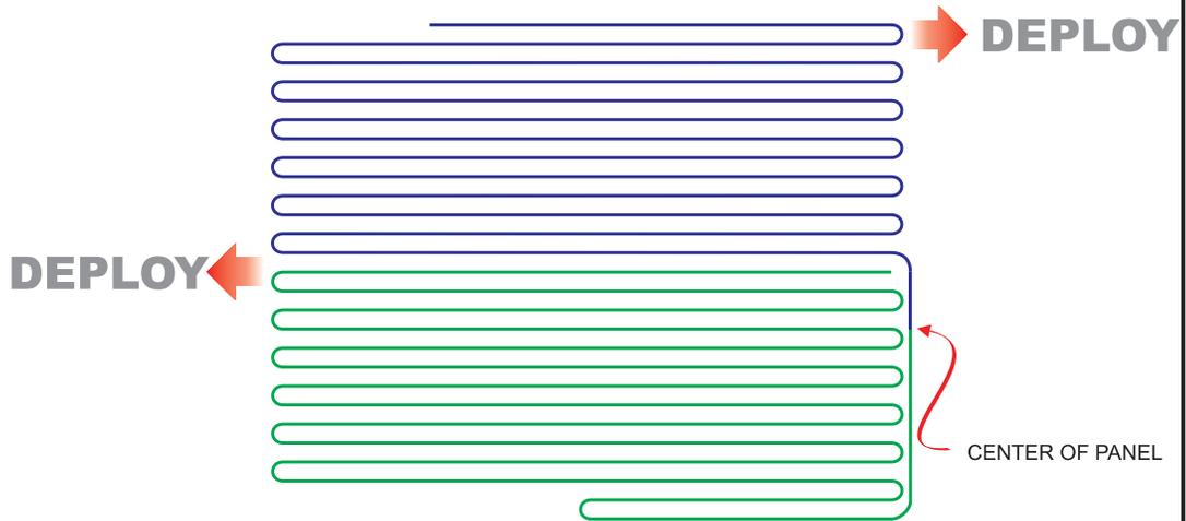
**EXAMPLE OF A 26 SHEET B-40 TANK LINER**
