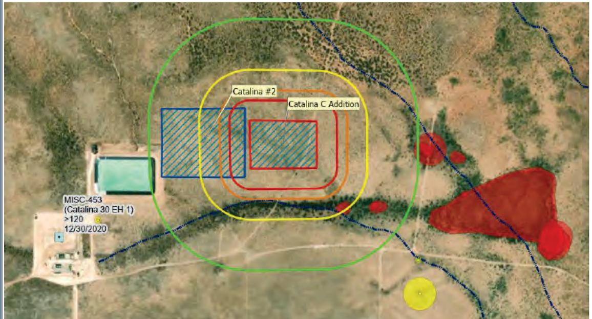
*The Catalina C Containment provides additional produced water storage for Tascosa Energy well stimulation programs. This image shows that a mapped watercourse is slightly more than 300 feet from the edge of the containment, depth to groundwater exceeds 120 feet in the auger boring MISC-453, and suspected and actual karst structures are more than 480 feet from the containment.*
