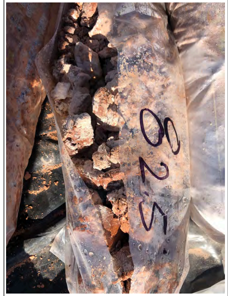
10. Closeup of core sample at 82.5 feet bgs
