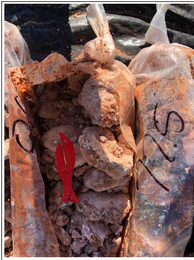
7. Core sample at 80 feet bgs
