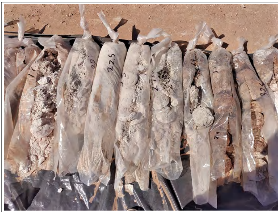
3. Core samples from 17.5 to 32.5 feet bgs
