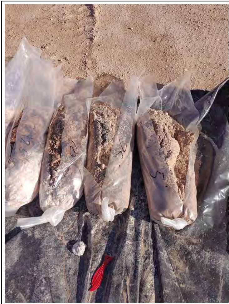
5. Core samples from 2.5 to 12.5 feet bgs
