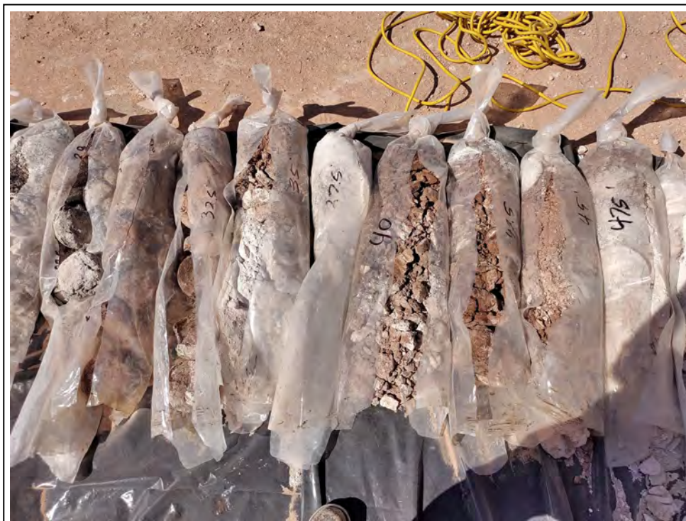
4. Core samples from 28.5 to 48 feet bgs
