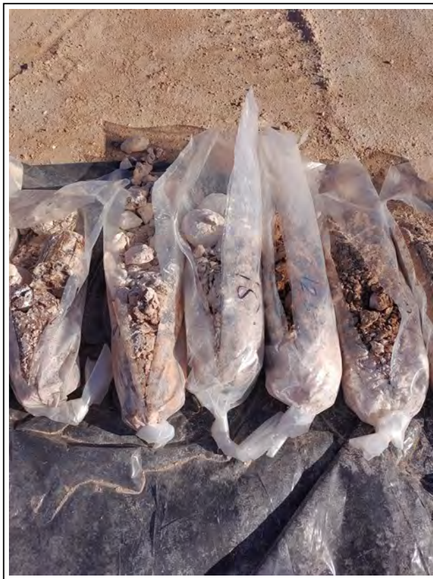
5. Core samples from 10 to 20 feet bgs
