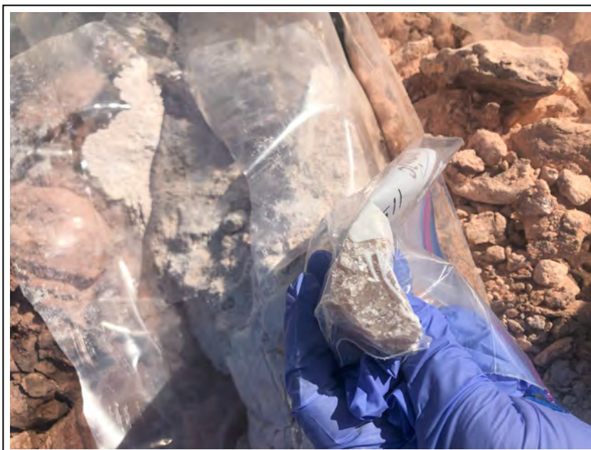
12. Anhydrite closeup at 115 feet bgs
