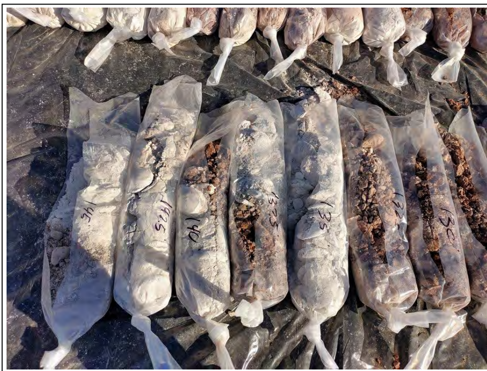
8. Core samples from 132.5 to 145 feet bgs
