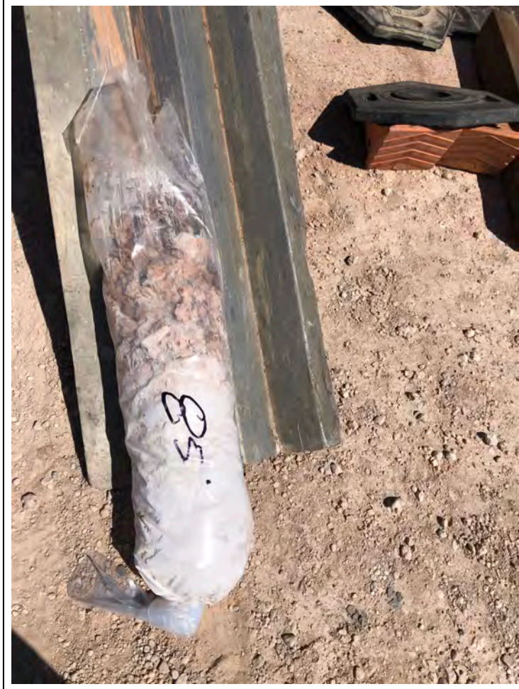
9. Core sample from 82.5 to 85 feet bgs
