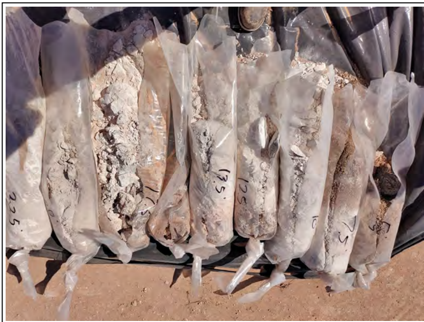
2. Core samples from 5 to 22.5 feet bgs
