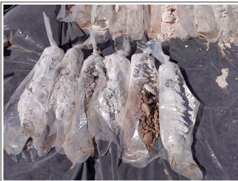
5. Core samples from 52.5 to 65 feet bgs
