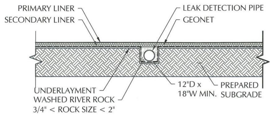
**SUMP LEAK DETECTION PIPE DETAIL**
