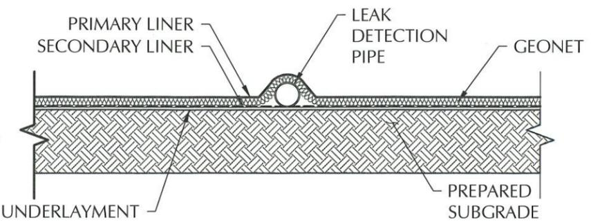
**SIDE SLOPE LEAK DETECTION PIPE DETAIL**
