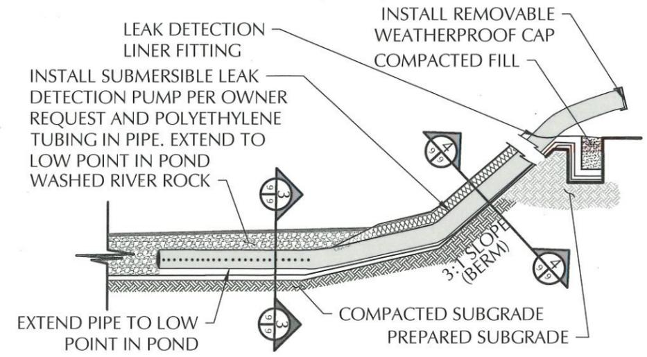
**LEAK DETECTION/SAMPLING SYSTEM DETAIL**
