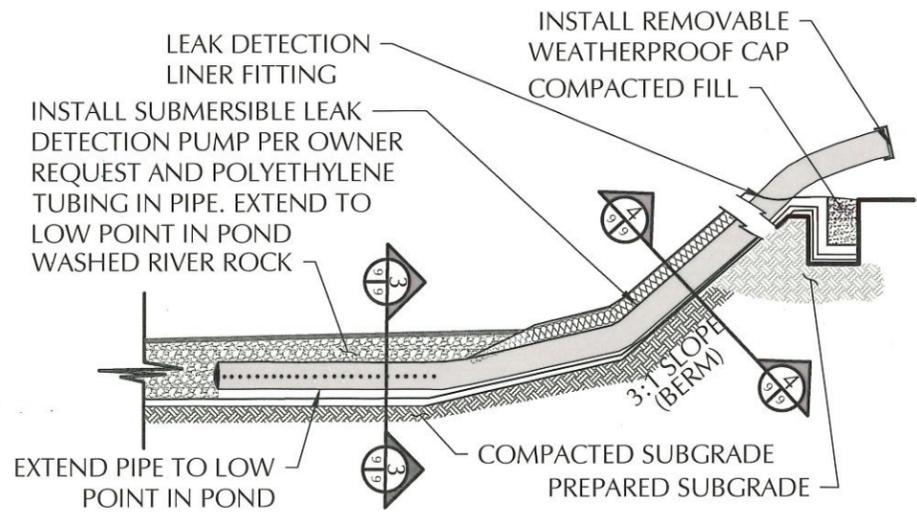
**LEAK DETECTION/SAMPLING SYSTEM DETAIL**
