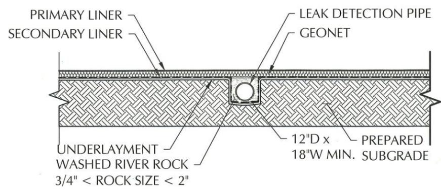
**SUMP LEAK DETECTION PIPE DETAIL**
