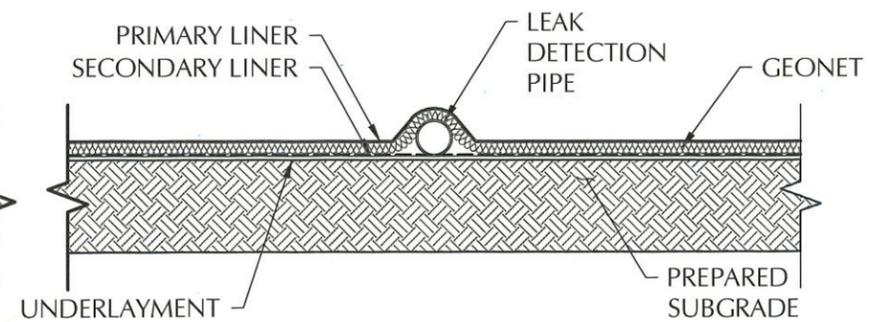
**SIDE SLOPE LEAK DETECTION PIPE DETAIL**
