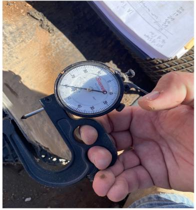
2022-10-14: Measurement of FML HDPE Liner Tie In
