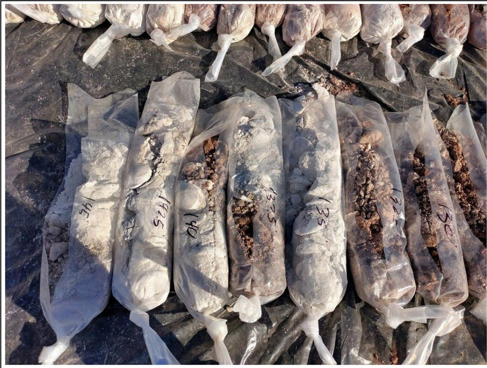
8. Core samples from 132.5 to 145 feet bgs
