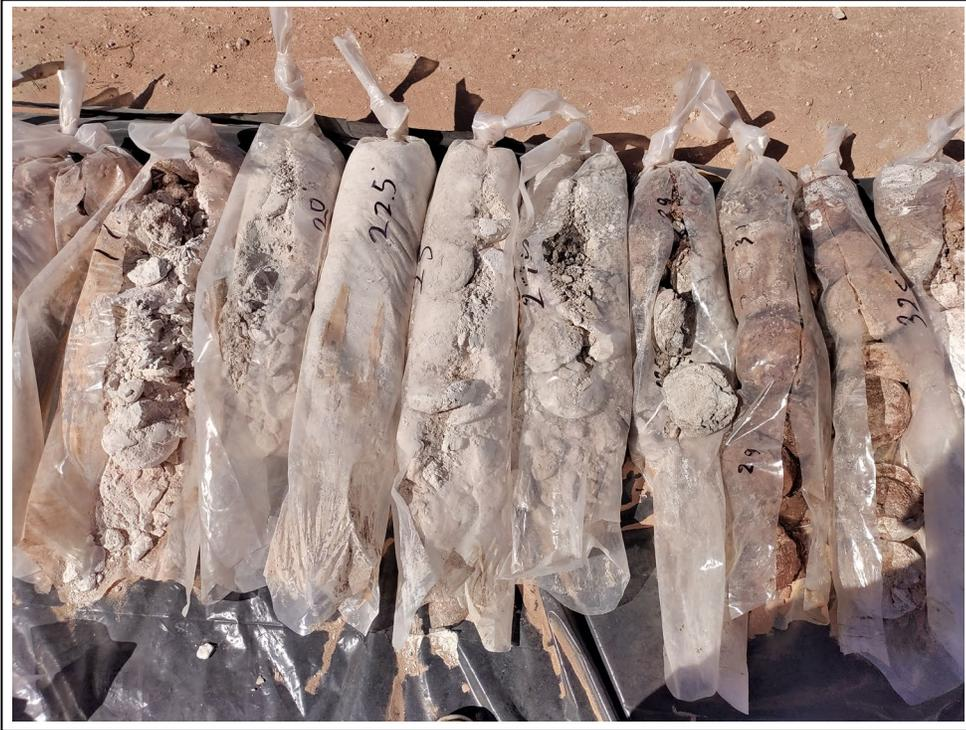
3. Core samples from 17.5 to 32.5 feet bgs
