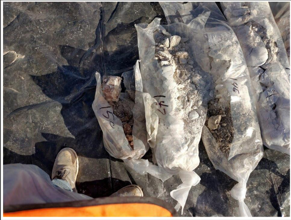
9. Core samples from 145 to 150 feet bgs
