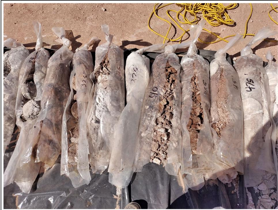
4. Core samples from 28.5 to 48 feet bgs
