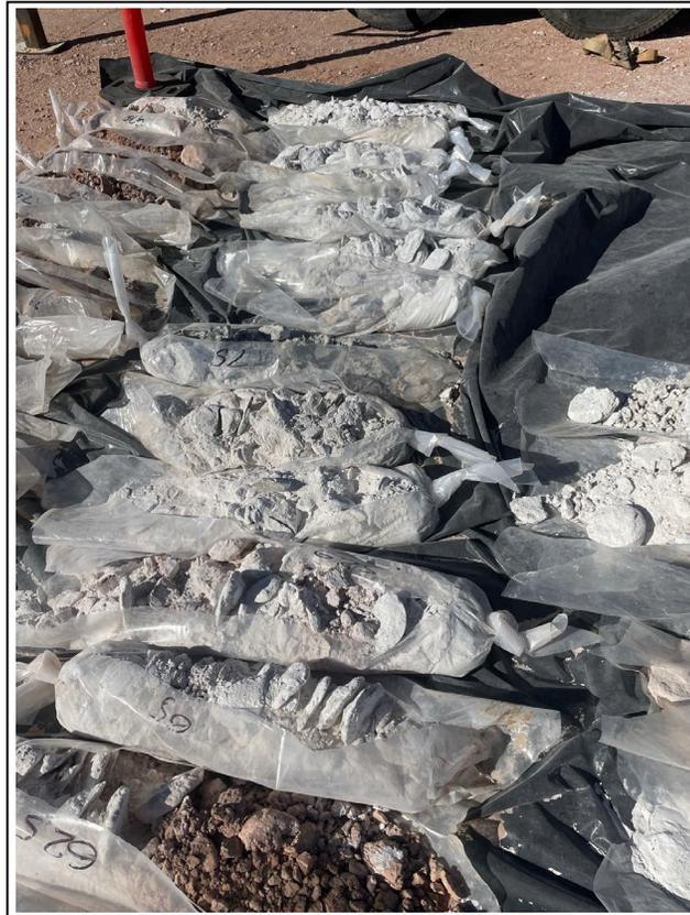
6. Core samples from 62.5 to 95 feet bgs
