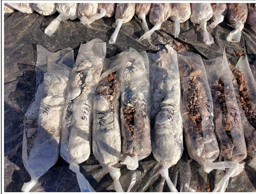
13. Core samples from 127.5 to 145 feet bgs
