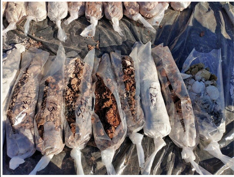
7. Core samples from 115 to 132.5 feet bgs
