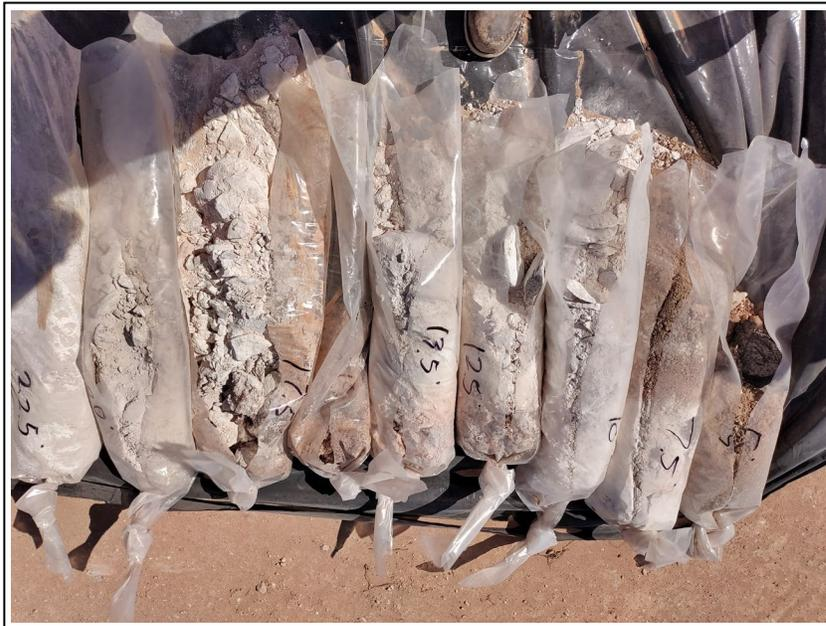
2. Core samples from 5 to 22.5 feet bgs
