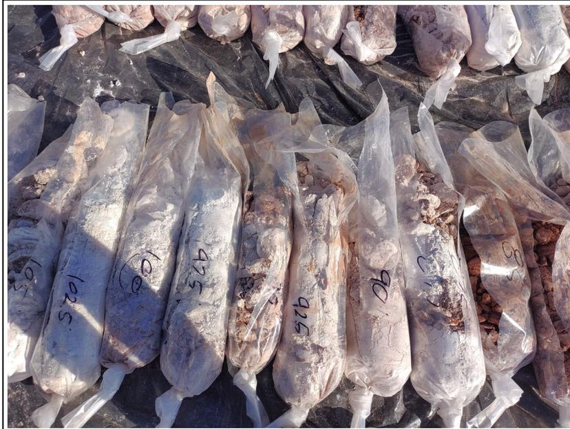
6. Core samples from 82.5 to 105 feet bgs
