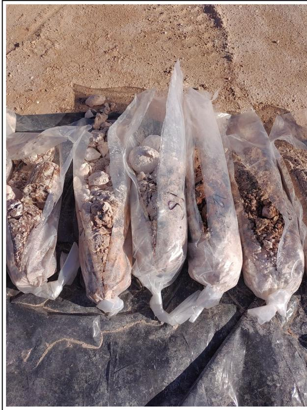
5. Core samples from 10 to 20 feet bgs
