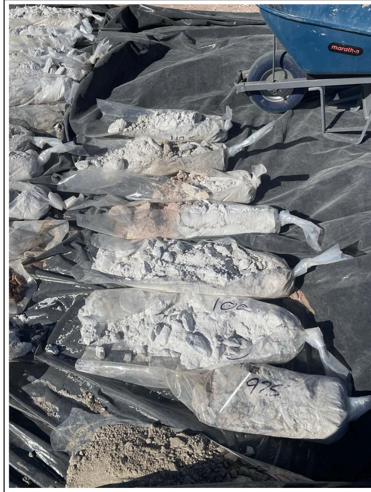
7. Core samples from 97.5 to 112.5 feet bgs
