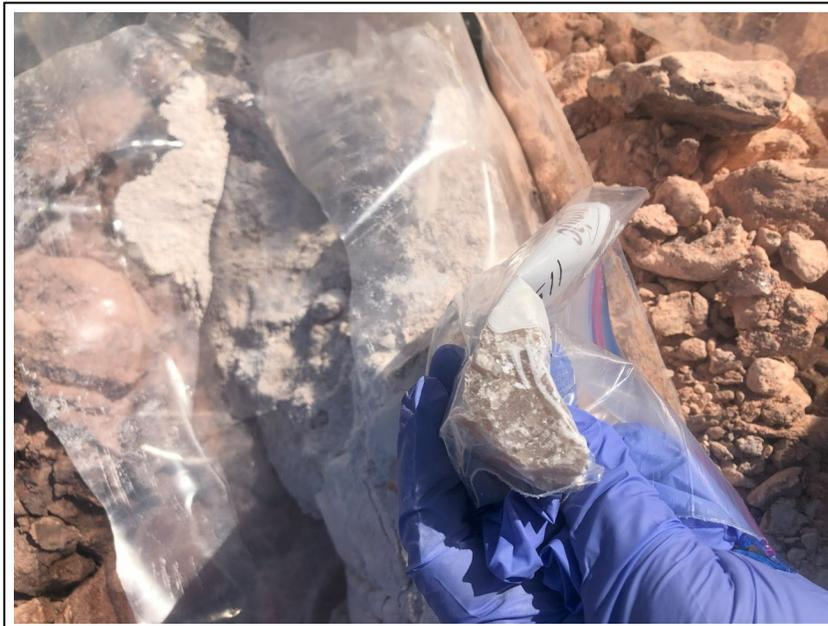
12. Anhydrite closeup at 115 feet bgs
