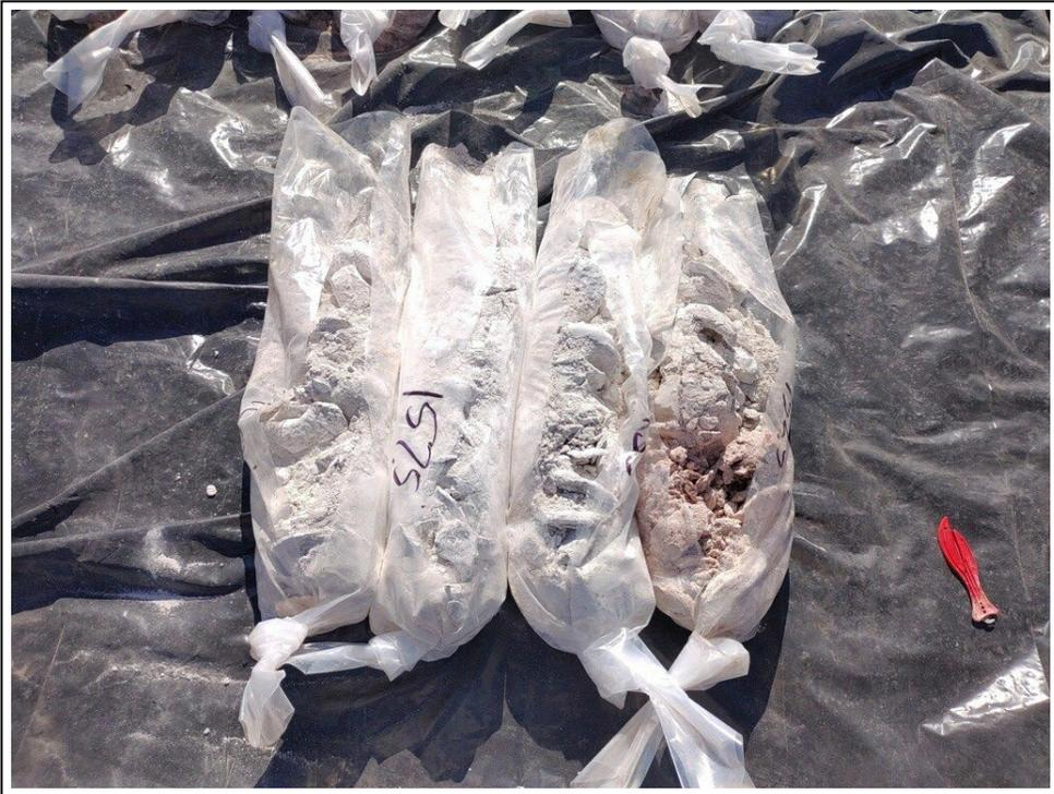
10. Core samples from 150 to 160 feet bgs
