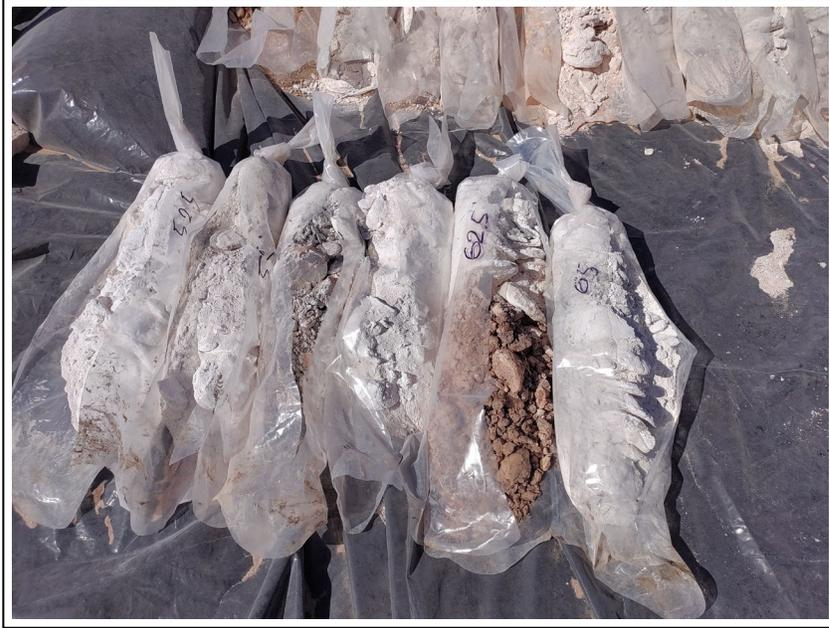
5. Core samples from 52.5 to 65 feet bgs
