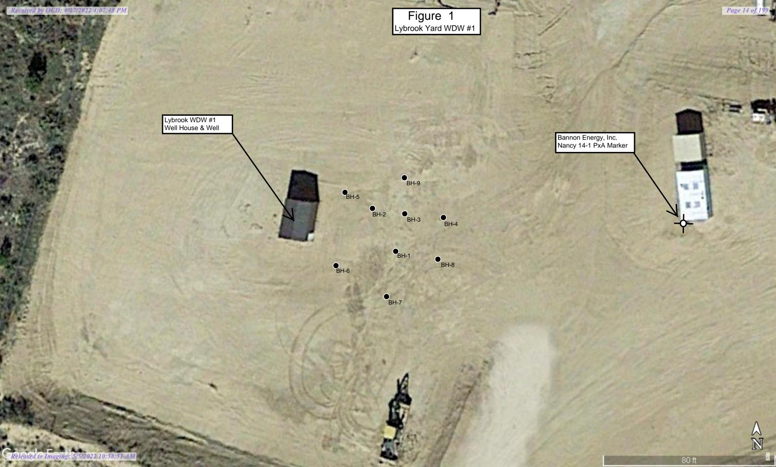
Page 15 of 199 Received by OCD: 4/27/2022 4:07:48 PM Figure 2 Lybrook WDW #1 Well house and Lybrook WDW #1 Remedial Excavation Approximately 30' x 20' x 18' Deep ●BH-9 ●<sub>BH-5</sub> BH-2 BH-4 ●<sub>BH-3</sub> Steel Injection Line ●BH-1 Communications Cable BH-8 ●BH-6 ●<sub>BH-7</sub> Approximate Extent of Remaining Soil Hydrocarbon Impacts [40' diameter, beginning at approximately 15' depth and extending to approximately 35' (about 930 CY)] N Released to Imaging: 5/5/2022 10:58:51 AM 60 ft
