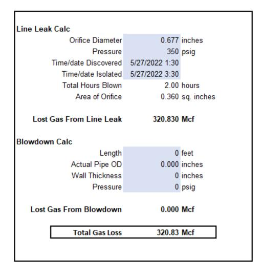
Lost Gas=(Orifice Diameter)^2\*Pressure\*Time Blown
