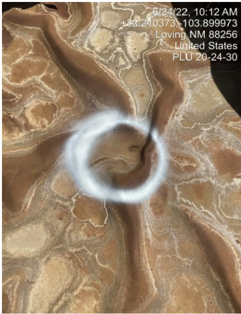
Photograph 1 Date: June 24, 2022 Description: View of tear in liner discovered during liner inspection.
