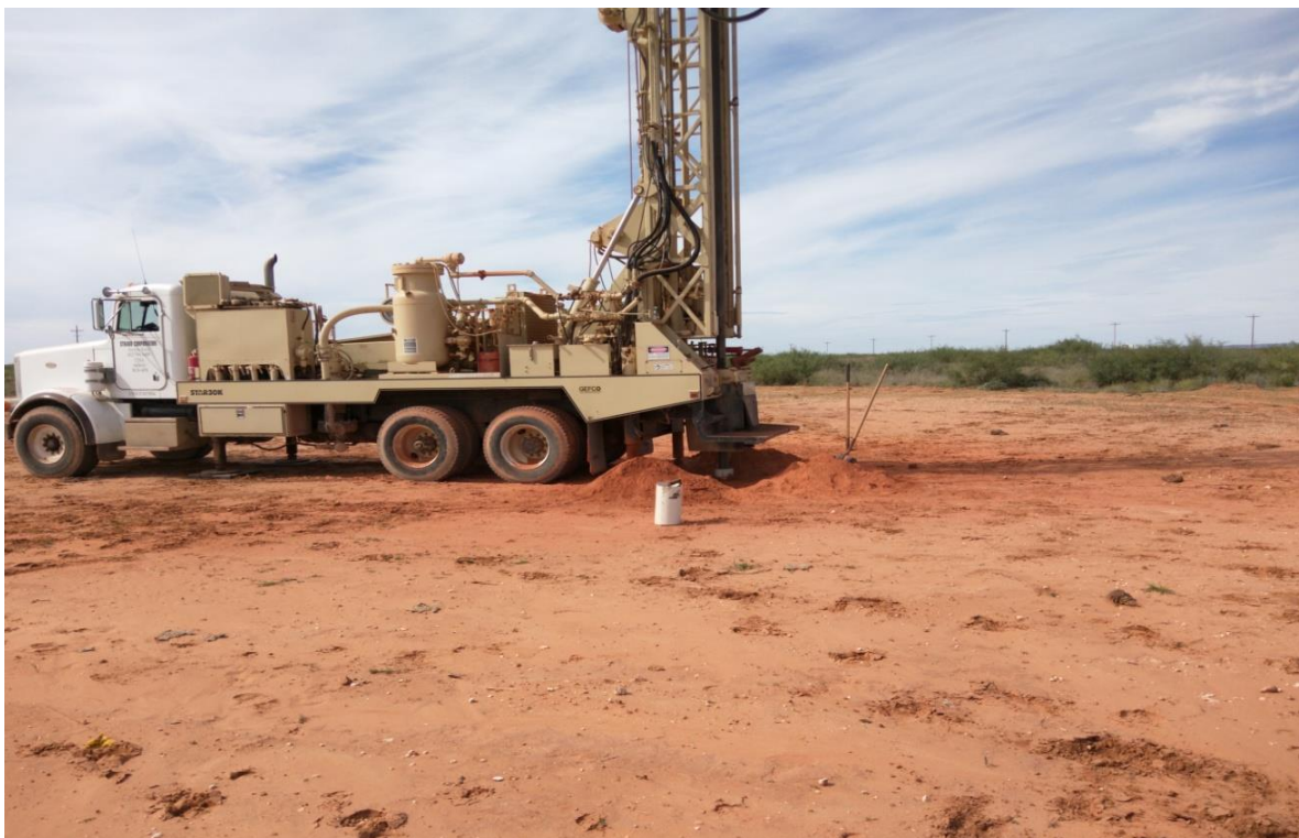
Palladium 7-1 4-Inch Poly – Advancement of Soil Boring SB-1
