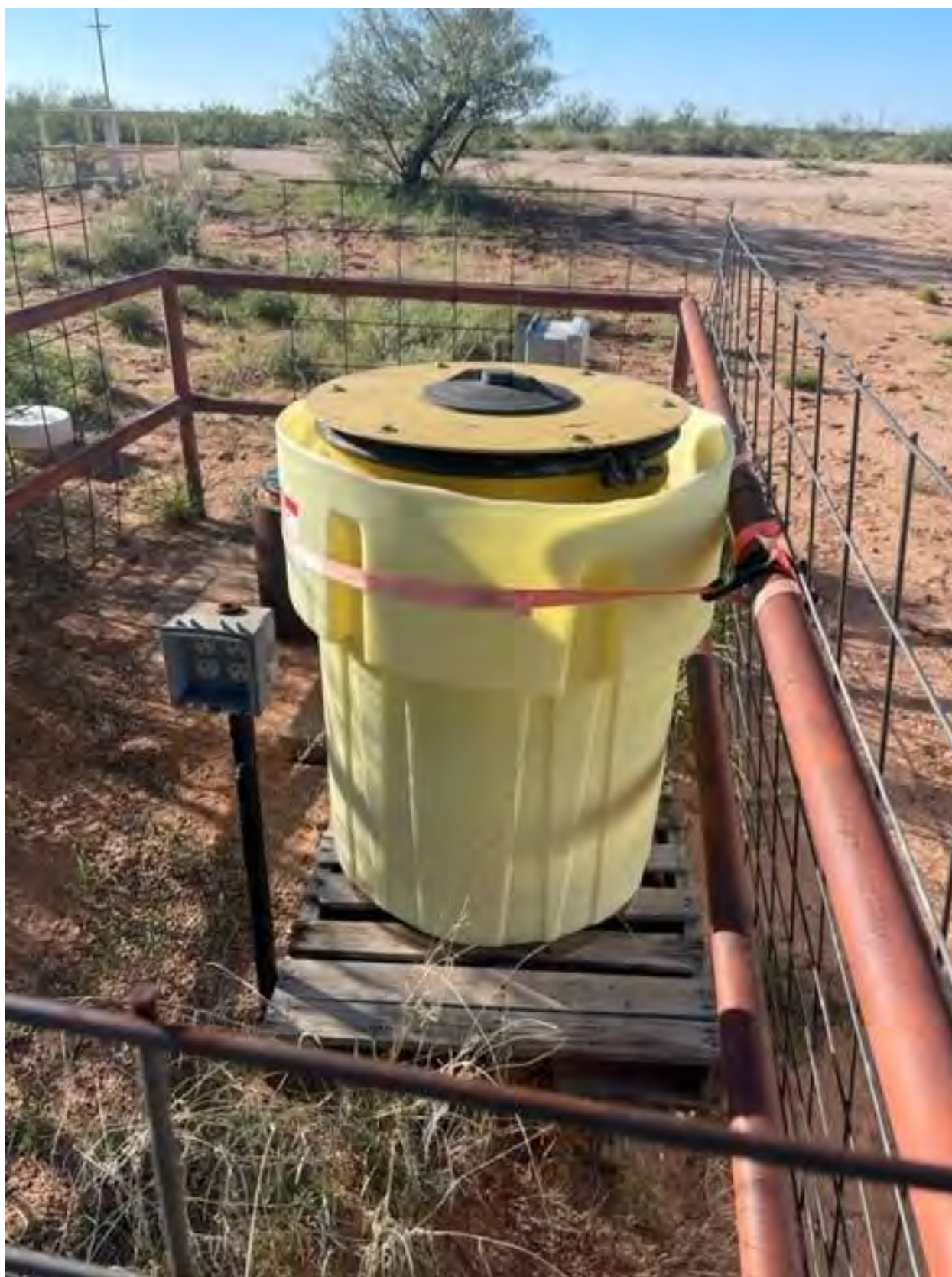
Jal #4 Gas Plant, Jal, New Mexico - Field-Deployed Drum in open overpack with Ventilated Barrel Cover – Successfully evaporates groundwater monitoring IDW purgewater “24-7”
