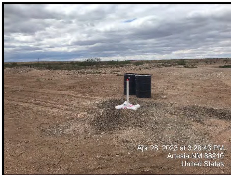
PHOTOGRAPH NO. 10 – A typical view of the April 2023 temporary monitor wells at the time of gauging on April 28, 2023.
